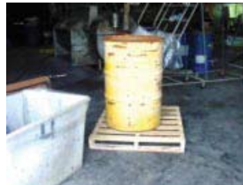
The 55-gallon drum contains the 32-gallon drum of hot sodium hydrosulfite and a quantity of coolant water.
